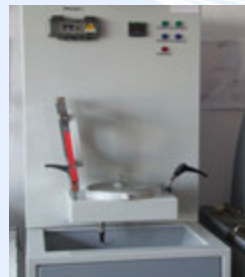
Fig. 82. Penetrometru BRANCA IDEALAIR, Italia
