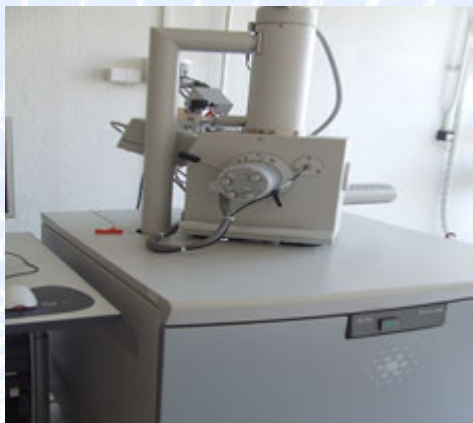
Fig. 69. Microscop electronic de scanare SEM/EDAX, Quanta 200-FEI Holland
